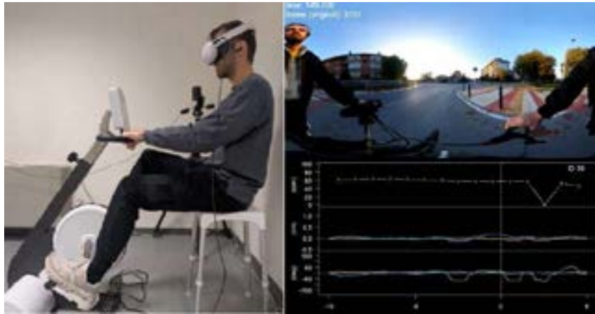
Figure 1: Left: Experimental setup. The participant pedalled on an exercise bike while viewing the 360° video. Right: video frame showing an approaching expected stop (top panel), with concurrent recordings of cadence (top trace) and head movements (middle and bottom traces). In this example, the participant briefly stops pedalling after the cyclist stops at the stop sign (vertical dashed line).
