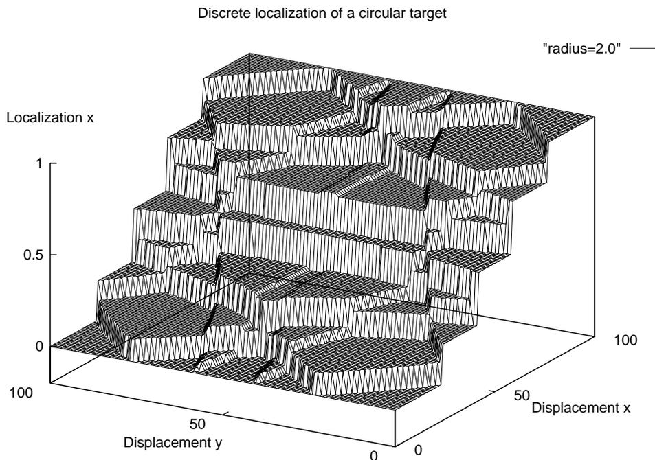
Figure 4: Simulation of target localization by discrete centroid calculation for a relative target diameter of 4 pixels (100 x 100 steps; "Localization x" in grid units)
