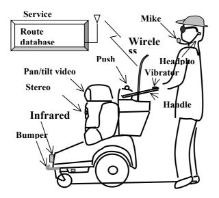
Figure 1. Configuration of RoTA.
