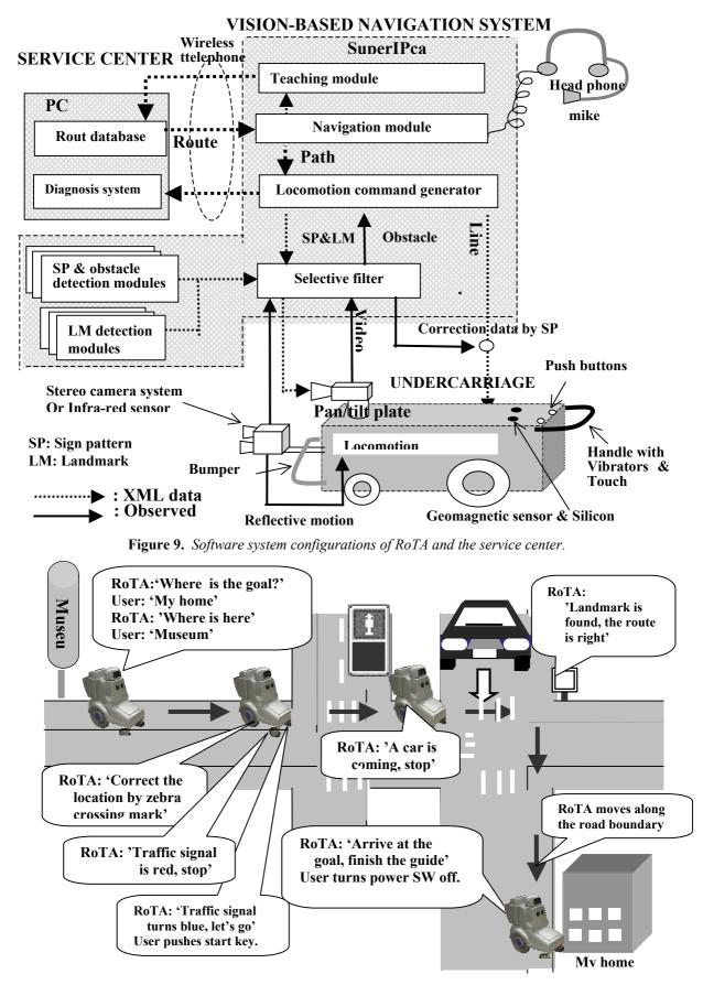
Figure 10. An illustration of the RoTA guide.
