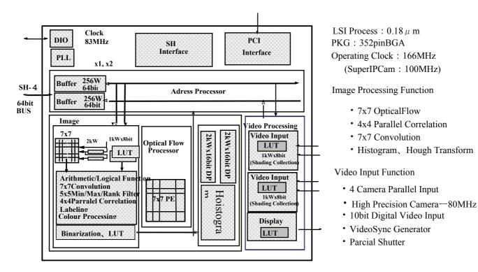
Figure 8. Super V chip configuration.
