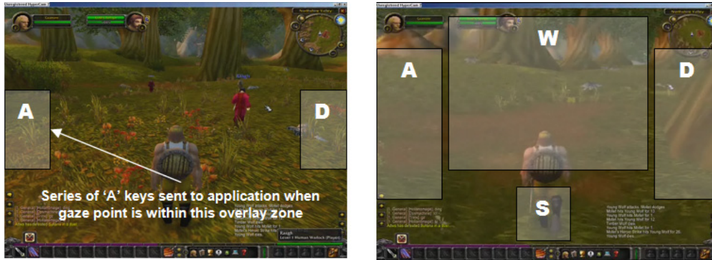
Figure 2. Screenshots showing Extended Snap Clutch being used with World of Warcraft . The 'no control' mode with overlay zones for rotating the avatar left and right (left); the 'locomotion' mode with overlay zones for moving and rotating the avatar (right).
