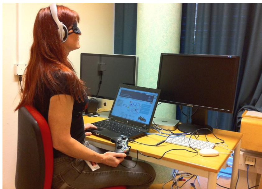
Figure 1. Test setup showing use of laptop touch pad for input and Xbox360 controller for output. Test subjects were blindfolded and wore ear protection.
